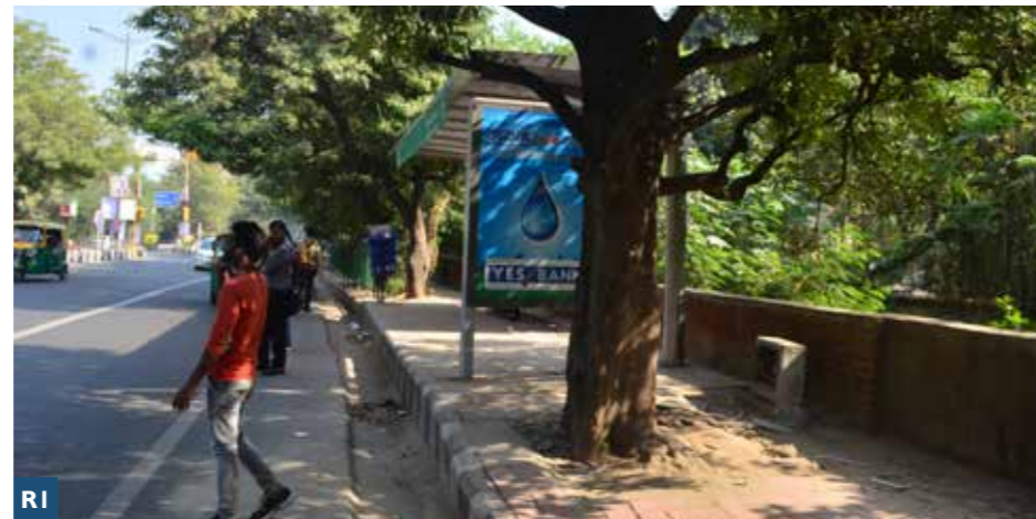
Bus stop covering almost the whole of Footpath width.
